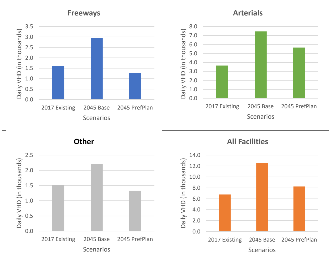
Figure 16: Daily VHD by Facility Type within the Palmdale Sphere of Influence for All Scenarios
